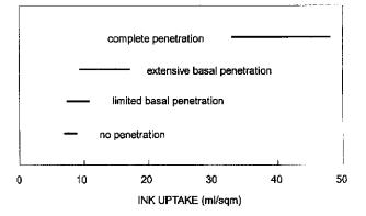
Figure 3. Liquid volume uptake for papers of different penetration characteristics
