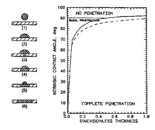
Figure 2. Theoretically calculated drop penetration modes for a thin porous medium simulating paper (Ref. 5)
